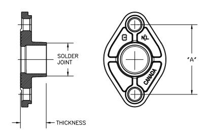
PARTS AND MATERIAL: FLANGE: CAST BRASS, NO LEAD ALLOY C89833 BOLT: STEEL, ZINC PLATED NUT: STEEL, ZINC PLATED GASKET: NEOPRENE
