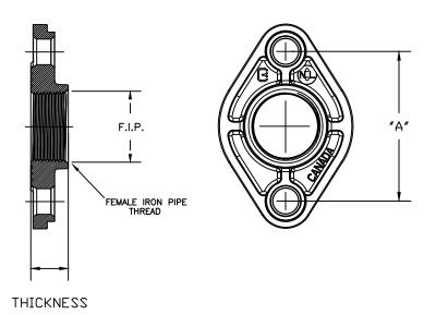
PARTS AND MATERIAL: FLANGE: CAST BRASS, NO LEAD ALLOY C89833 BOLT: STEEL, ZINC PLATED NUT: STEEL, ZINC PLATED GASKET: NEOPRENE
