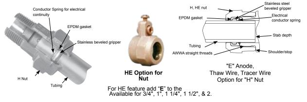
NOTE: H, B, GJ, J, K nuts have the same threads and are interchangeable.
